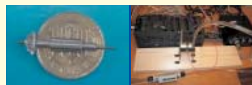
Fig.3 8mm turbine rotor with (left) and experimental setup for performance measurement (right).
